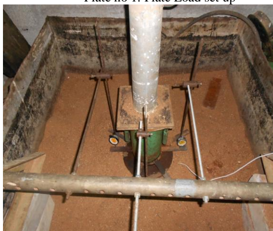
Plate no 1: Plate Load set up
